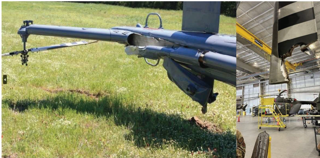
Damage to tail rotor assembly (Tab S-13)
