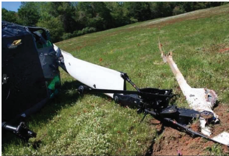
MRH separated from transmission upon impact with ground (Tab S-12)
