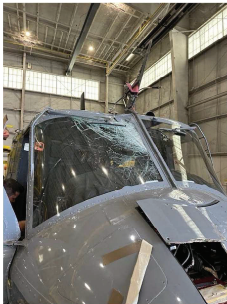
Damage to Cabin Nose Section (Tab S-10)
